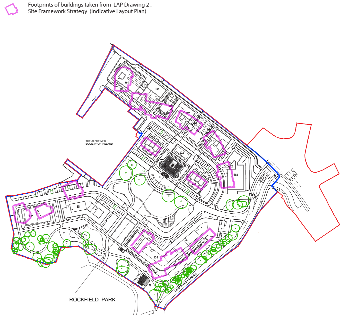
LAP Overlay - LAP Indicative Layout Plan overlaid on proposed development layout plan.
